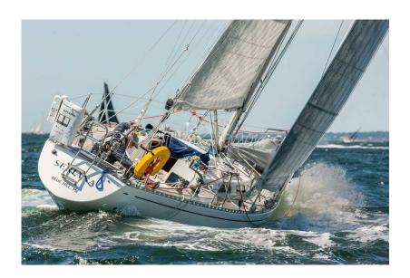
**The boat moved well** due to its long waterline and narrow form, with relatively deep entry. I sailed with a removable inner forestay with staysail and 155 percent ap genoa on the roller furler. I used the genoa extensively, including reaching in strong winds and downwind in strong winds wing and wing using the spinnaker pole. I have a removable bowsprit 1' beyond the bow to get beyond the stanchions.
