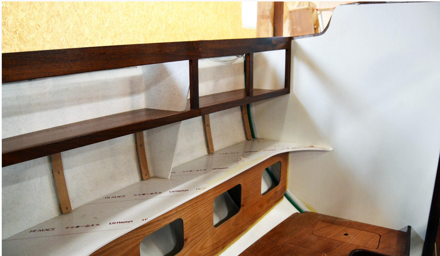
Port side settee with lots of cupboards and stowage
