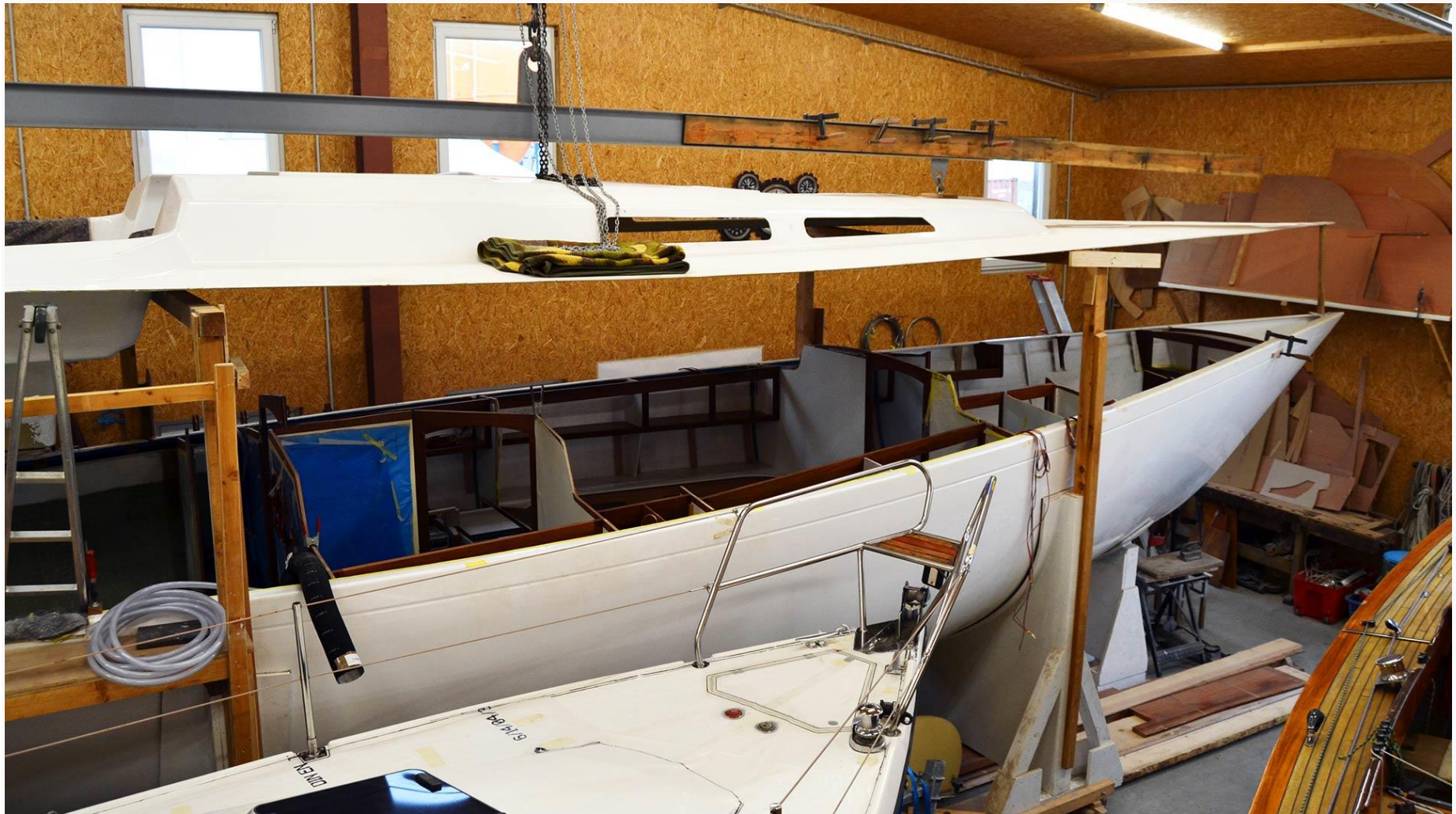
Hull #1 with deck superstructure shortly before marriage
