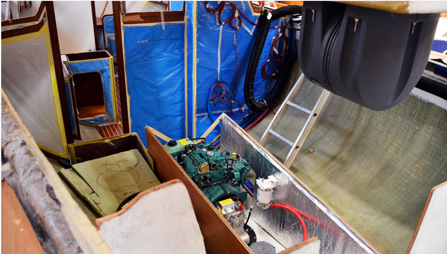
30 hp Volvo-Penta on a sail drive
