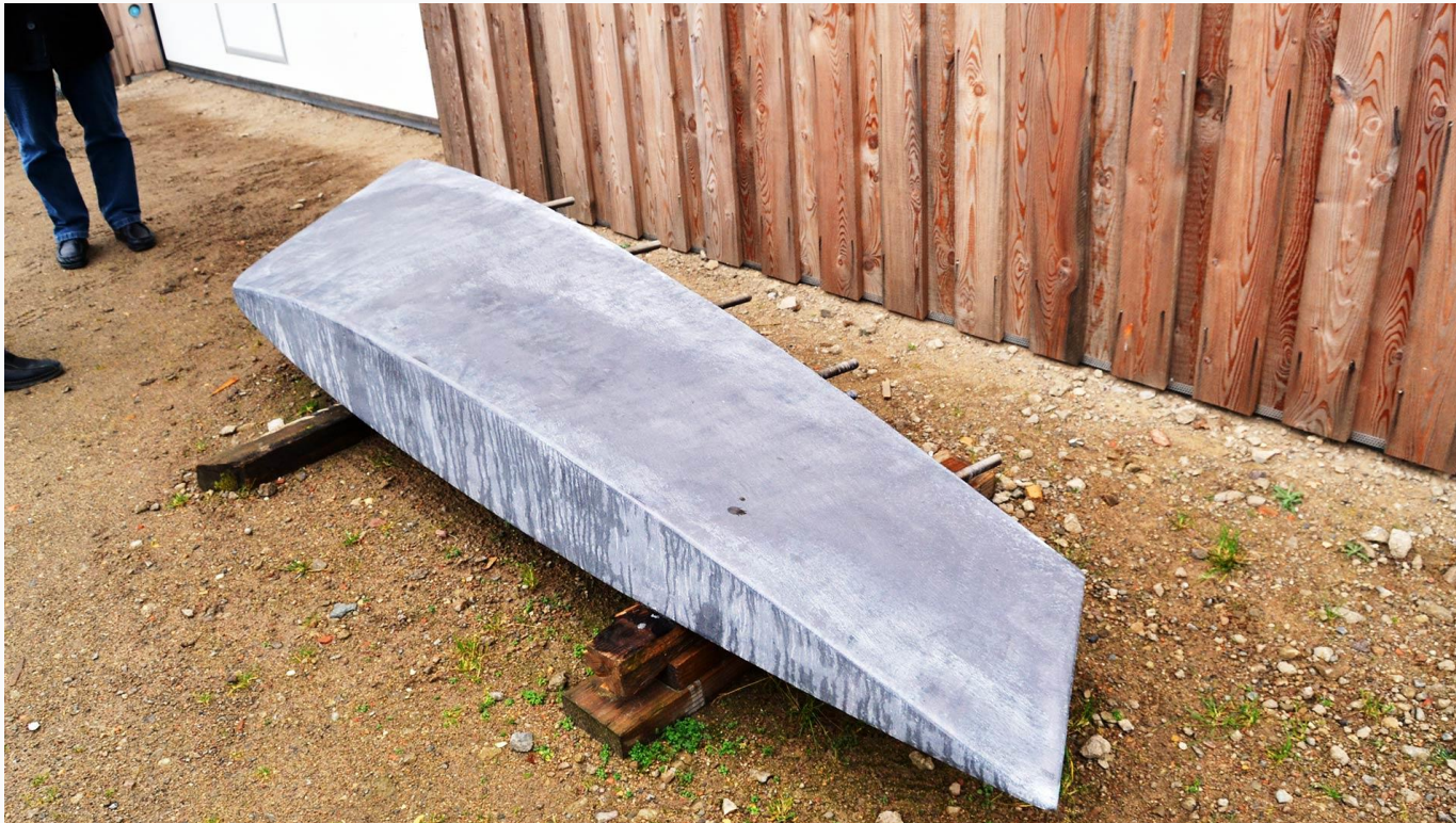
3.75 tons of pure lead. The keel of the OMEGA 42
